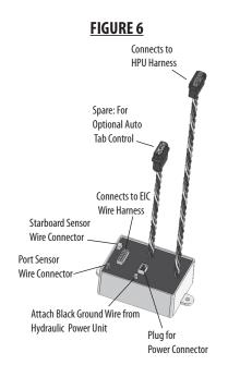
**Power Cable:** Attach the black wire to 12 volt negative ground and the orange wire with inline 20 amp fuse to 12 volt positive source and plug into EIC Relay Module. Power source must be capable of supporting 20 amps.
